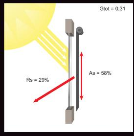
Rs: Solar reflectance As: Solar absorbance Gtot: Solar factor, fabric + glazing
